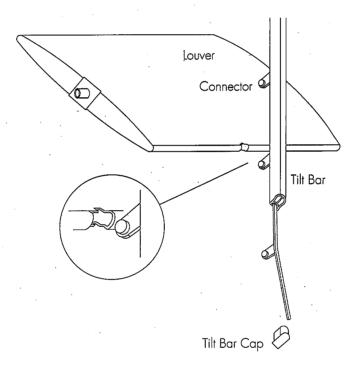
Note: It is possible to re-insert the tilt bar connectors without damage. Simply hold the louver, place the connector in the notch and press firmly. It is not necessary to remove the tilt bar.
