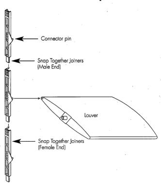
Note: The top and bottom joiners in a panel are shorter. Replace these joiners with the same type joiners.
