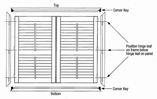
2. Insert the plastic corner keys into the ends of the top and bottom frames.
